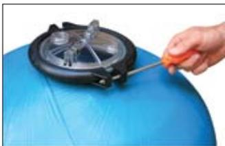
7. a. Attach the air release valve into the tank lid. **DO NOT OVERTIGHTEN AS THIS CAN DAMAGE THE TANK LID.**
